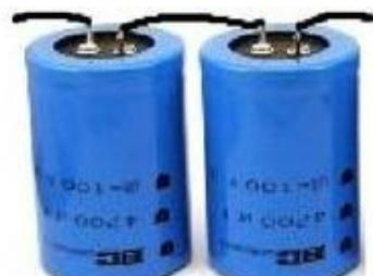
$$\frac{1}{C} = \frac{1}{C_1} + \frac{1}{C_2} + \frac{1}{C_3}$$
