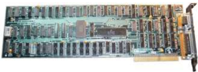
Monochrome Display Adapter (MDA) (1981)
